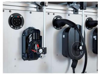
Test System for 1 to 10 entire AC wall boxes with outlet Type 2
