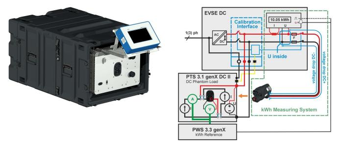
The PTS 3.1 genX DC can simulate any positive or negative flowing DC power by injecting DC voltage between DC+ and DC- path (0  $\dots$  1000 V) and DC current in the path with the current measurement element (0  $\dots$  600 A) separately into the EVSE DC. In this way up to 600 kW can be simulated with a few kW.
