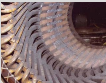
Stator rub due to eccentricity
