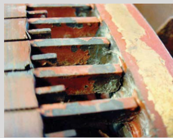
Broken rotor bar
