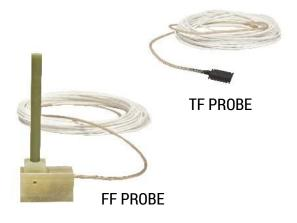
The Iris Power TFProbe™ and Iris Power FFProbe™ measure the air gap flux rate of change to detect shorted rotor winding turns in synchronous motors, hydrogenerators, and turbine generators. The probes, when connected to the portable Iris Power RFAII™ instrument, the Iris Power FluxTracII™ continuous monitor, or the Iris Power GuardII™ monitor with Flux Add-On, allow the user to monitor the health of motor and generator field windings on-line, periodically or continuously.
