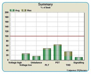
The PQ Secure automatic report generator provides comprehensive reports in accordance with a variety of norms like EN 50160, IEC 61000-2-2 etc.
