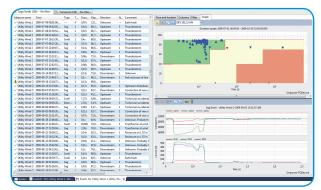
Evaluation of voltage sags with norm classification according to different standards and planning levels.
