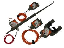
AmpLiteWire and VoltLiteWire sensors for voltage and current measurements on high voltage potential up to 40 KV and currents up to 2000 A.
