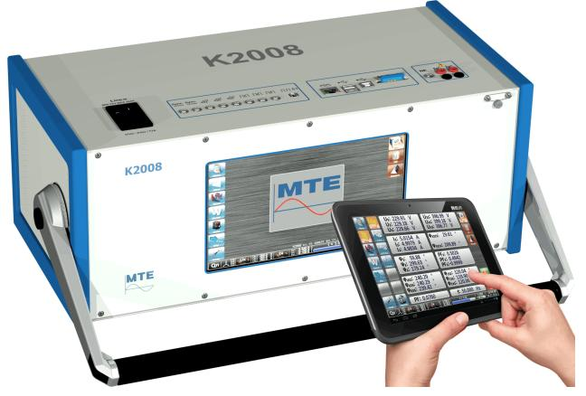
K2008 is a three-phase comparator of accuracy class 0.005 (50ppm) with direct voltage and current inputs. It has been designed for universal laboratory and test applications and is intended for checking and the calibration of reference standards for electrical power and energy. In addition, it can be integrated into meter or reference standard test systems of highest accuracy.
