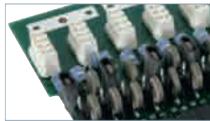
Version with LSA connection for use as patch panel version in new installations.
