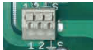
Conductor terminals for fast connection without tools (DBX TC 180).
