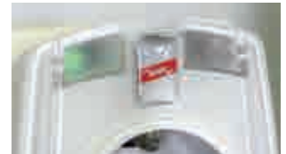
Visual operating state and fault indication of the power side (230 V).
