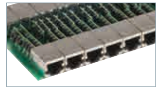
Version with RJ45 sockets shielded on both ends.
