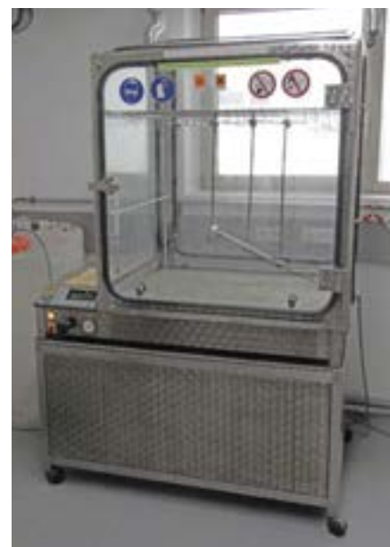
Figure 2: Test in a Kesternich chamber.
