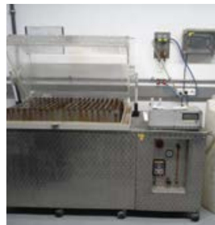
Figure 1: Test in a salt mist chamber.
